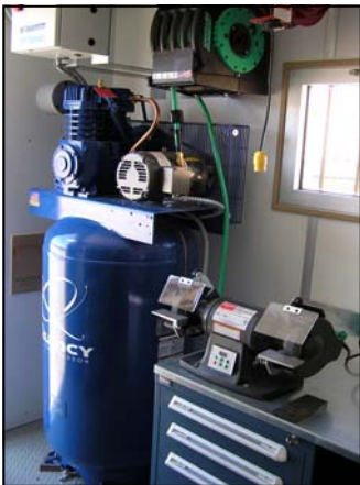
80 gal. compressor and variable speed grinder
